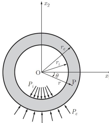
$$\sigma_{rr} = \frac{1}{r_e^2 - r_i^2} \left( r_i^2 P_i - r_e^2 P_e + \frac{r_i^2 r_e^2}{r^2} (P_e - P_i) \right)$$
